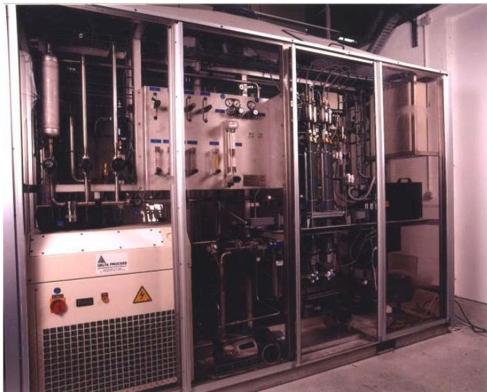
First automated system, installed at Moissy-Cramayel (France) for ensuring Kr and Xe very high-level purification. A whole factory building is now dedicated to such rare gas purification and the process is fully computer-control, working 24/24. A similar factory has been put up in Germany.
