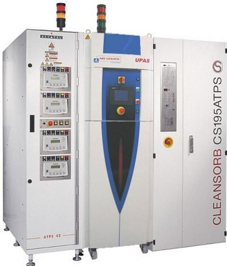
More advanced greenhouse gases remediation system commercialized under UPAS (Universal Plasma Abatement System) by Air Liquide company for microelectronics fabs at different locations in the world. It can handle up to 4 production plasma reactors (total gas flow up to 120 slm). Maximum MW power consumption 6 kW. From left to right, system computer controlled, surfaguide plasma abatement system, alkaline-bed unit for collecting process residue (scrubber).
